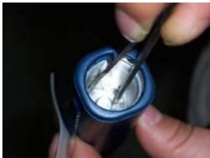
8. Replace the silicone shock-absorption pad, the battery, and the battery cap. If the reader makes a long beeping sound with LED flashing, it means the reader is resetting itself. Please wait for one minute then test to see if the reader is working. If it is working normally, please calibrate its time using the software before further usage.
