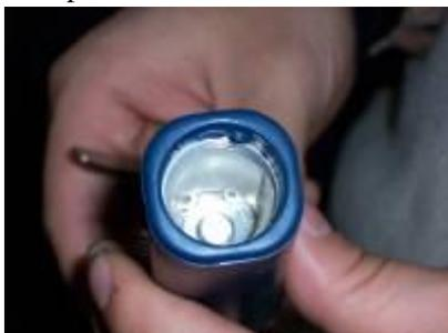
6. Remove the silicone shock-absorption pad from the inside wall of the battery compartment. (Be sure to replace it after the completion of this process.)
