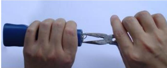
4. The battery cover is opened. Please note the location of the silicone-waterproofing ring. If the ring is damaged during the battery replacement process, please replace it with the spares provided. In addition, please note that the cathode (negative end) of the battery is facing outwards.
