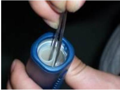
7. Create a circuit between the round metallic contact on the bottom of the compartment and the compartment wall for approximately 2-5 seconds.
